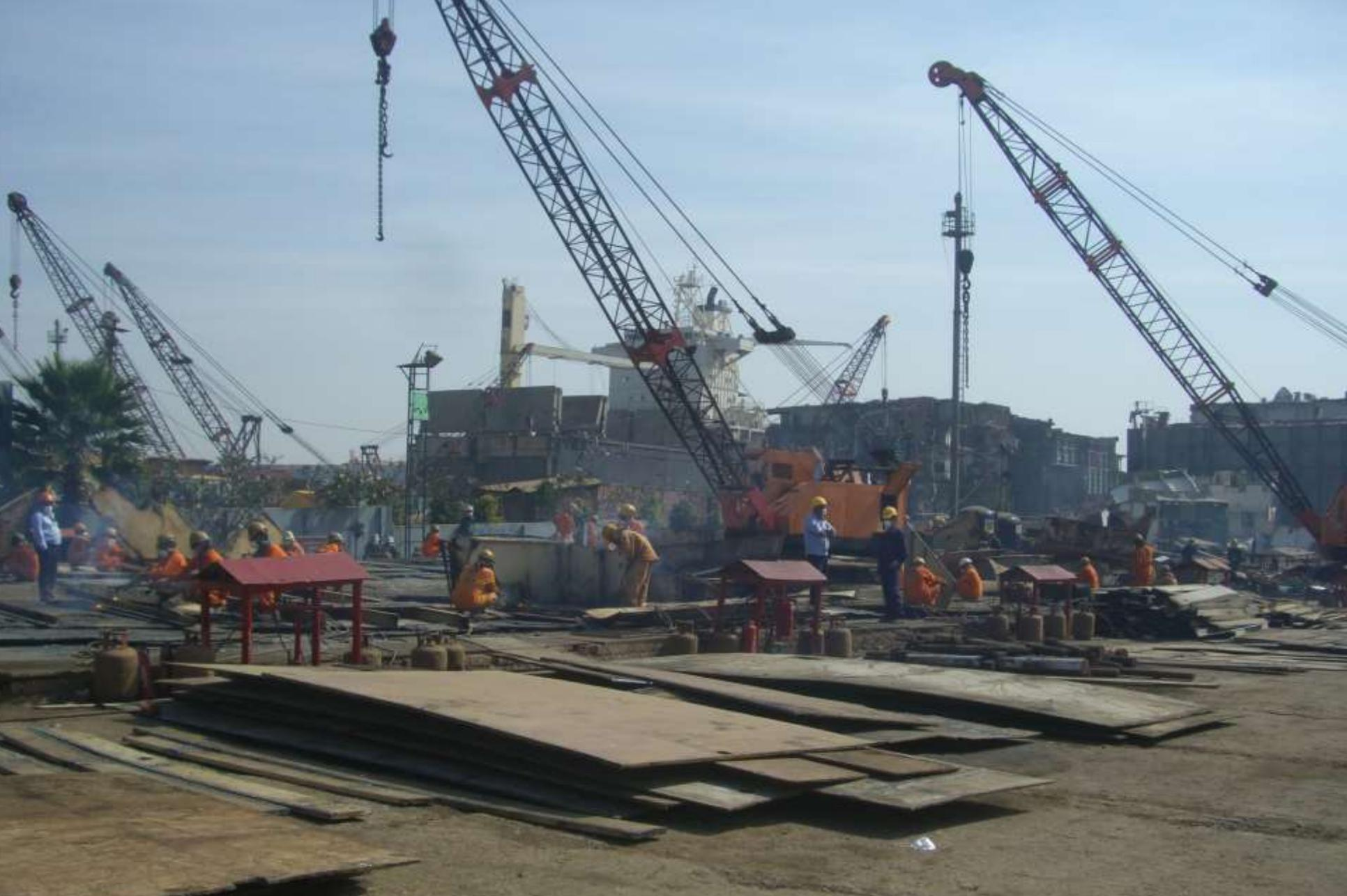
**Secondary cutting on concrete to avoid soil contamination**
